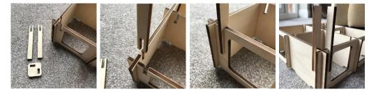
Once a pair of leg pieces are in place fit the "foot" onto the end. It will be a snug fit onto the end of the legs but just align the holes with each leg and wiggle each side downwards a little at a time until the foot is level with end of the leg, or even a small amount further on.
