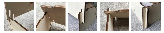
Continue to slot each wall piece together until 3 outer walls are constructed. When you get to the final outer wall piece you will be slotting it into the two other sides at the same time. Please "wiggle" (technical term) each side down a little at a time so that the final piece stays horizontal, rather than trying to push one side fully down.
